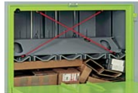
Robust: The twofold guided press ram
