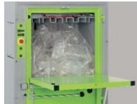
Compaction of plastic material (foil)
